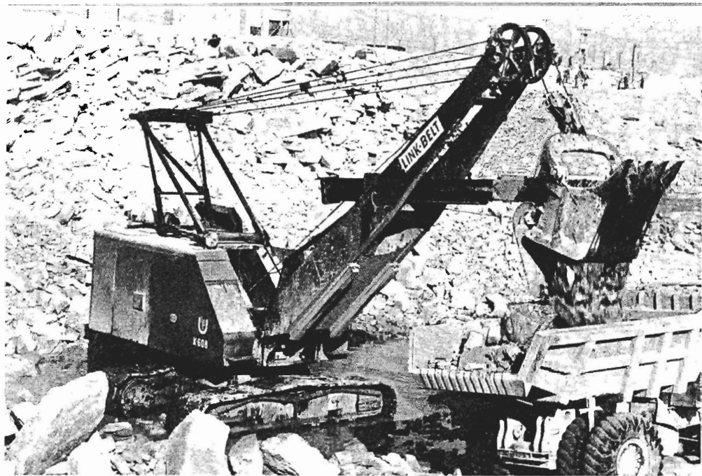
BIG REACH, BIG PULL, BIG BITE — The 3-yard K-608 series hoe has the reach, weight and power for deep digging and tough jobs.
