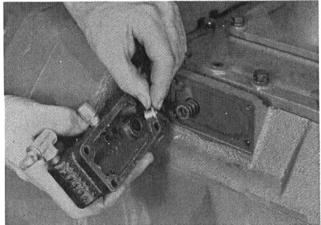
16. Remove the hat-type sleeve from the bore in the valve.
