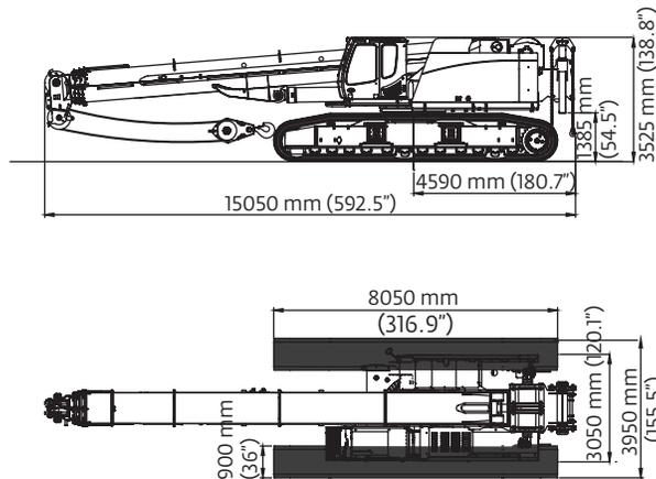
Transport weight: approximately 49 060 kg (108,156 lb) (with two hoists, 8 m (26 ft 3 in) boom extension, 60 t (66.1 USt) hook block, no side frames, and no counterweight)
