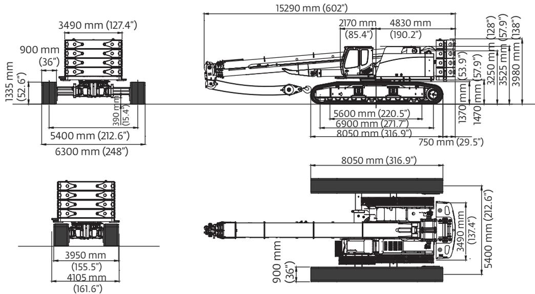
Operating weight: approximately 80 460 kg (177, 382 lb) (with two hoists, 8 m (26 ft 3 in) boom extension, 60 t (66.1 USt) hook block, 900 mm (36 in) triple bar shoes, and no counterweight).
