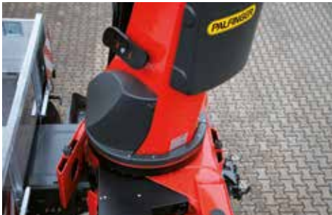
CONTINUOUS SLEWING SYSTEM UNRESTRICTED MOVEMENT
