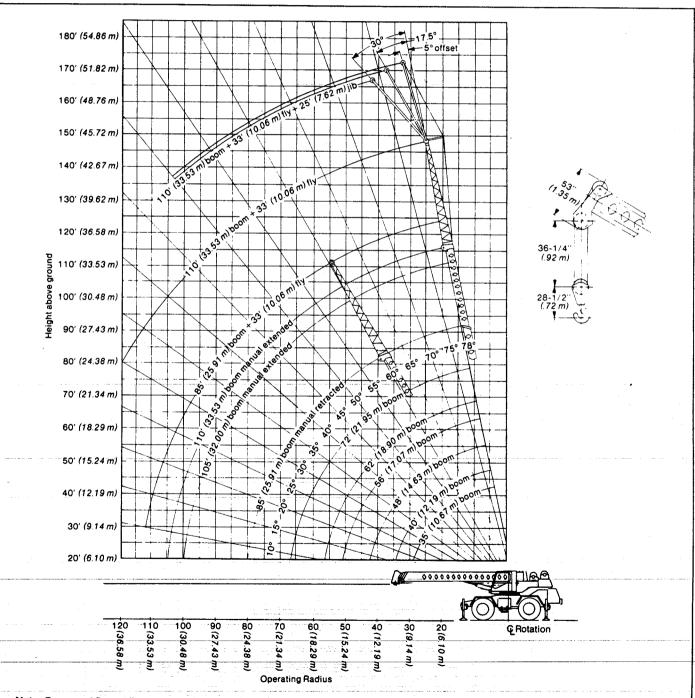
Note: Boom and fly and jib geometry shown are for unloaded condition and machine standing level on firm supporting surface. Boom deflection and subsequent radius and angle change must be accounted for when applying load to hook.
