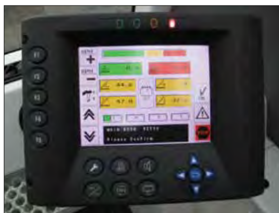
State-of-the-art, user friendly rated capacity limiter provides continuous feedback of crane lift and position data.
