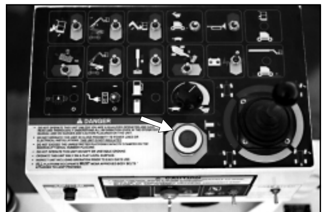
Platform control box Emergency Stop switch location.
