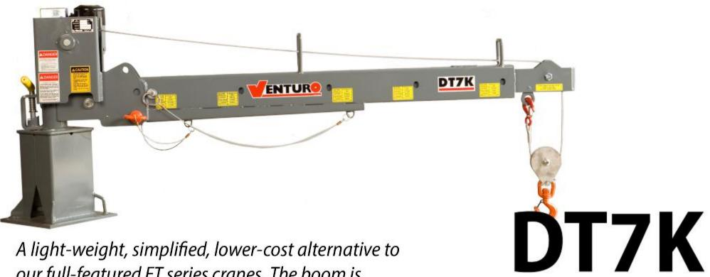
A light-weight, simplified, lower-cost alternative to our full-featured ET series cranes. The boom is manually telescopic from 6 to 10 ft. and features a 3-position manual boom elevation system with the weight of the boom spring counterbalanced for quick, one-handed raising and lowering.
