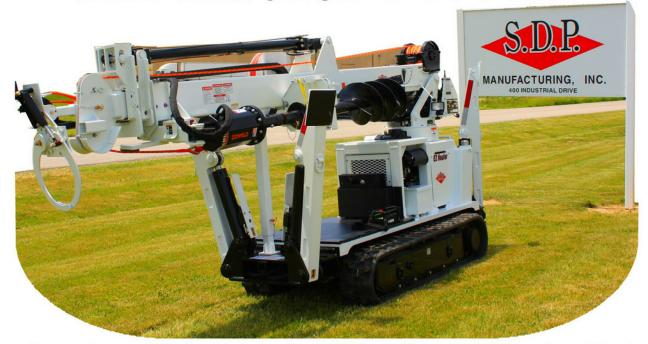
3400 lb Capacity. Overall, length Including Crane is 15 ft. Automatic Sensing with Alarm Capable of 20 degree Side to Side and Front to Rear Travel Angle
