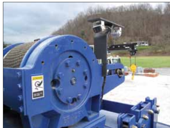
Conveniently positioned cameras display the winch as well as the blind area directly behind the crane. Full color video display in operator cab is standard equipment.
