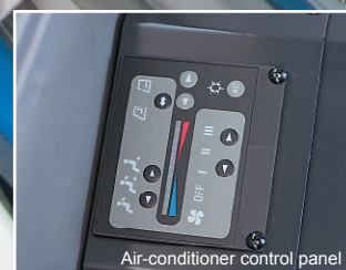
Air-conditioner control panel
