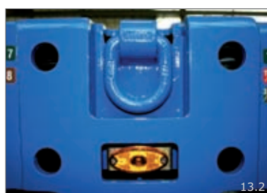
Solid attachment points for load securing - With side marker lamps protected in the outer frame
