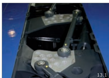
Steering rods protected between main beams
