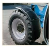
**FENDERS**Streamlined, rugged fenders provide increased protection from mud and debris.
