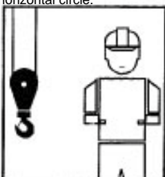
RETRACT BOOM - (Telescoping Booms) Both fists in front of body with thumbs pointing inward.
