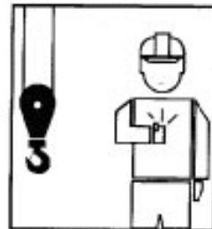
RETRACT BOOM - (Telescopic Booms) - One Hand Signal. One fist in front of chest, thumb pointing outward and heel of fist tapping chest.
