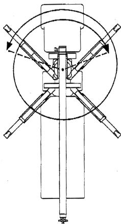
Pioneer Cranes utilizes the "X" outrigger design and goes one step further. Instead of just 375 degrees of rotation, Pioneer gives the operator a full 500 degree boom rotation. This truly allows working over the front of the unit with no compromise. Compared to other manufacturers, Pioneer gives you full stability and total access to the job site, It's a tough combination to beat.
