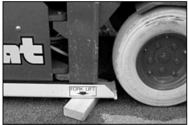
Figure 8.13—Pothole Protector Interlock Test
