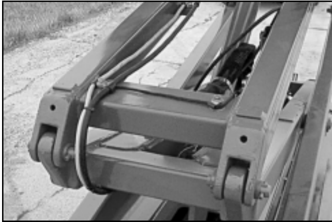
Figure 8.5—Cables and Wiring Harness
