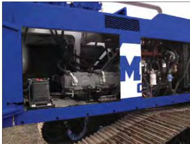
Large access doors, spacious machinery compartments simplify preventative maintenance and service of the crane.
