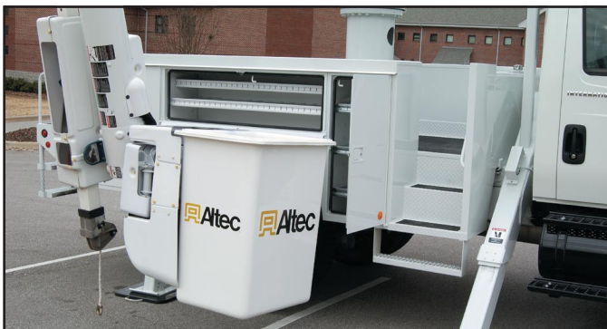
125 degrees of lower boom articulation allows operator to access bins and the ground from the non-overcenter position.
