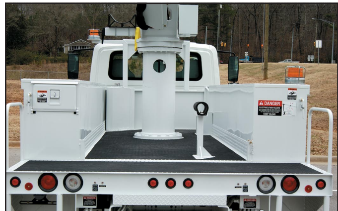
Select the normal upper boom stow position for open bed space or the low stow position to simplify platform access.
