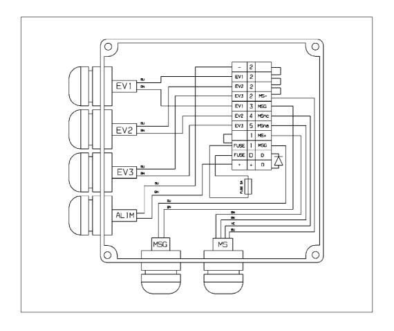
Electric schematic for crane - mercury slope sensor - seat box
