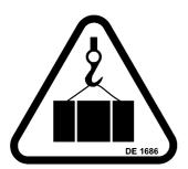
It is absolutely prohibited to walk or stop under a suspended load and for unauthorized persons to be within the working area.
