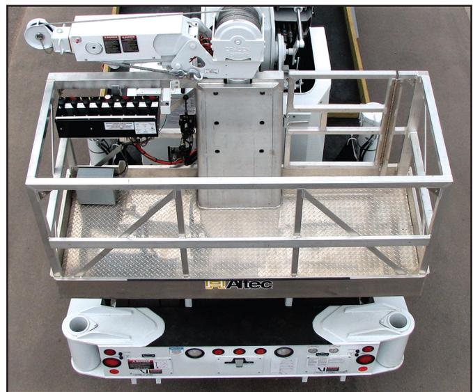
Hydraulically extendible jib may be manually rotated on its base and pinned in 5 working positions. Jib pinned perpendicular to upper boom (90°) is capable of lifting at maximum capacity, while located out of the way of operators inside the platform.
