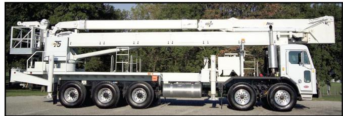
When folded in the road travel position on commercially produced chassis, the AH150 is 44.75 ft (13.64 m) in length, 13.3 ft (4.05 m) in height and meets the legal weight requirements, including bridge formula, in most US states.
