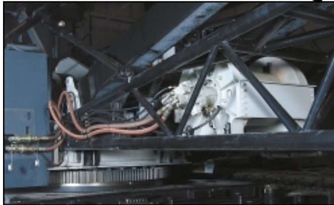
Optional third hoist drum is mounted in boom base section.
