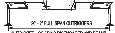
OUTRIGGER LOCK PINS DISENGAGED AND BEAMS AT FULL HORIZONTAL EXTENSION
