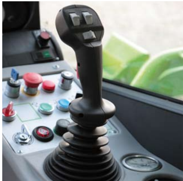
◀ Roto MCSS models are equipped with an electronic multi-functional joystick, placed on the adjustable armrest (photo left). Optionally, a second joystick can also be installed on the left armrest. Roto 600 and 400 series are equipped with a simpler electro-mechanical proportional joystick (photo above).
