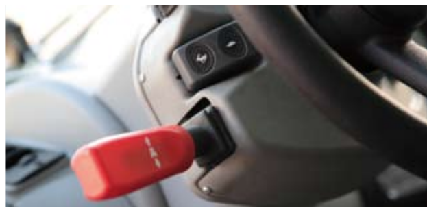
▶▶ A column-mounted Finger-Touch electrical control lever allows the driver to reverse driving direction without taking his hands off the steering wheel. The high/low travel speed range selector is electrically controlled via push-buttons on the Roto MCSS (photo right) or a rocker switch on Roto 600 and 400 series models (photo above).
