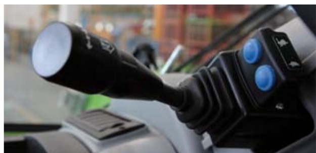
▶▶ A column-mounted Finger-Touch electrical control lever allows the driver to reverse driving direction without taking his hands off the steering wheel. The high/low travel speed range selector is electrically controlled via push-buttons on the Roto MCSS (photo right) or a rocker switch on Roto 600 and 400 series models (photo above).
