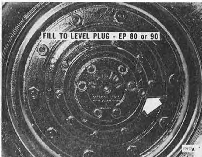
Figure 71 PLANETARY DRIVE LEVEL PLUG (CLARK)
