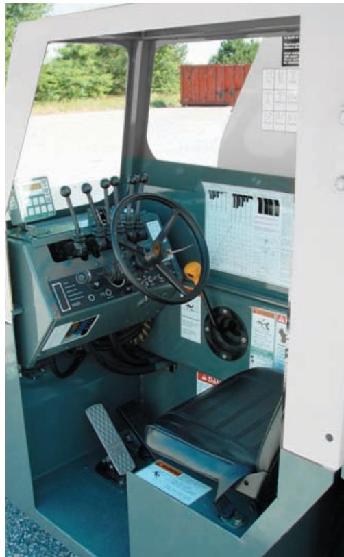
**Standard:** Open air cab shell w/overhead safety glass
