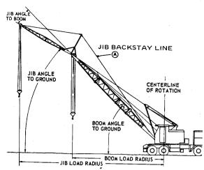
length listed in the lifting capacity chart deduct 400 lbs. from the capacity shown for the longest boom length for the radius required in (b).
