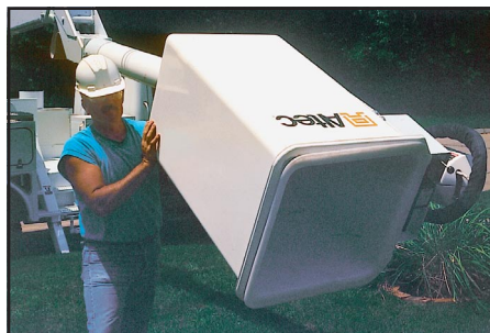
Quick Release Pin For Easy Tilting of Platform
