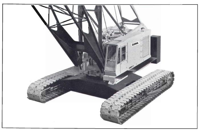
**TRUCK BASE:** The truck base is of all welded construction with axles designed to bolt to the side frames. The swing gear, and the anti-friction swing circle are integral with the truck base.
