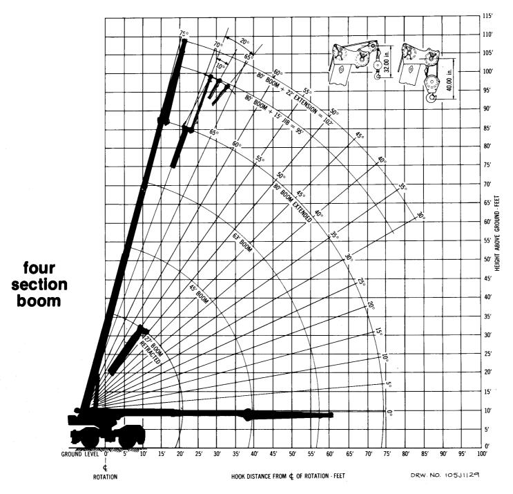
WARNING: Do not exceed 90 ft. load radius with erected boom extension or jib or a tipping condition will occur.
