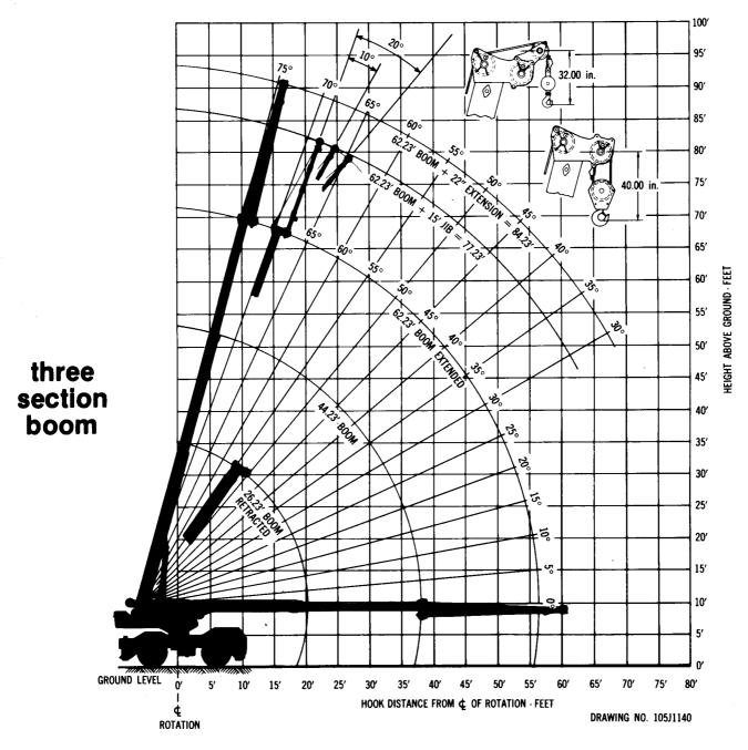
WARNING: Do not exceed 74 ft. load radius with erected boom extension or jib or a tipping condition will occur.
