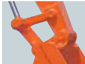
● Boss lubrication to bucket pins
