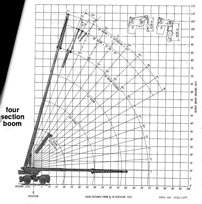
WARNING: Do not exceed 90 ft. load radius with erected boom extension or jib or a tipping condition will occur.
