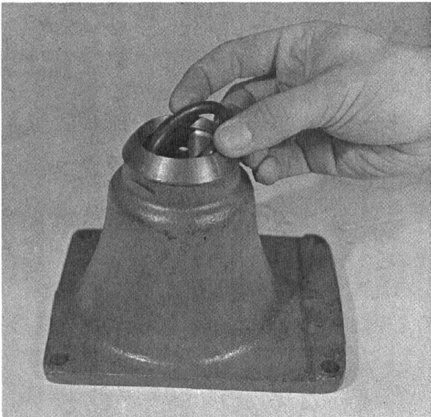
1. If so equipped, install the O-ring in groove in the housing.
