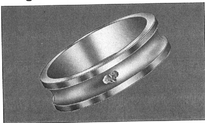
Figure 1. Raceway metal breaking down causing flaking or spalling.
