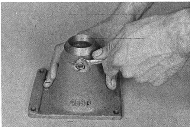
2. Install the lockwasher and nut to secure the pivot pin.
