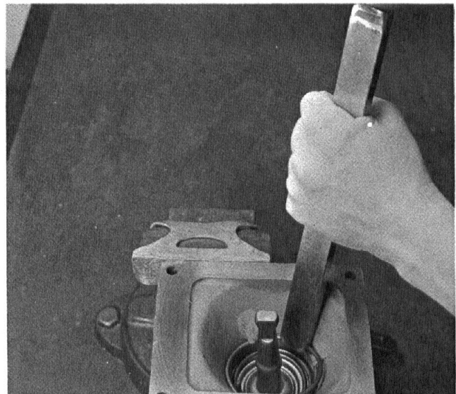
5. Seat the tension spring under the lugs in the housing.
