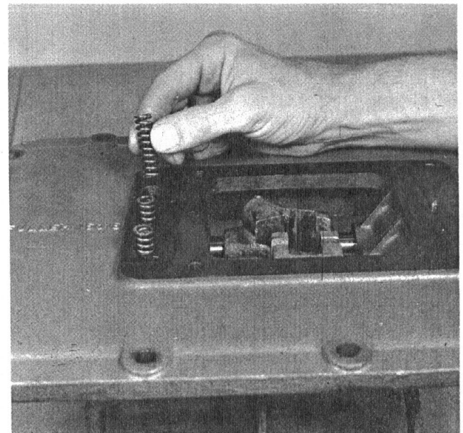
8. Install the tension springs on top of the balls in the bores.
