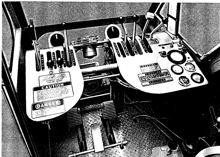
Operator control console
