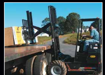
Lift capacity is 5000 lbs. at 24" load center
