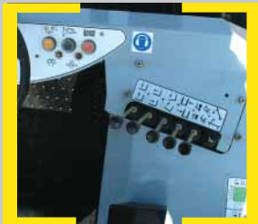
4-way mode enabled via hydraulic lever.
