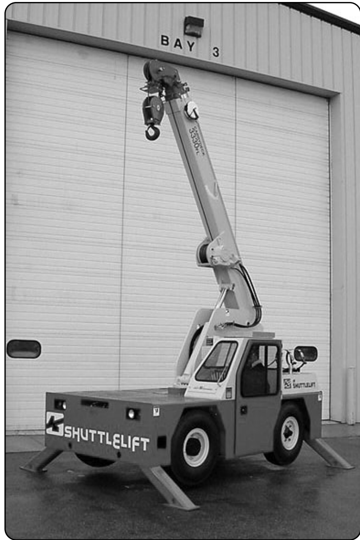
Single stage outriggers for operation in confined areas. Shown with optional cab.
