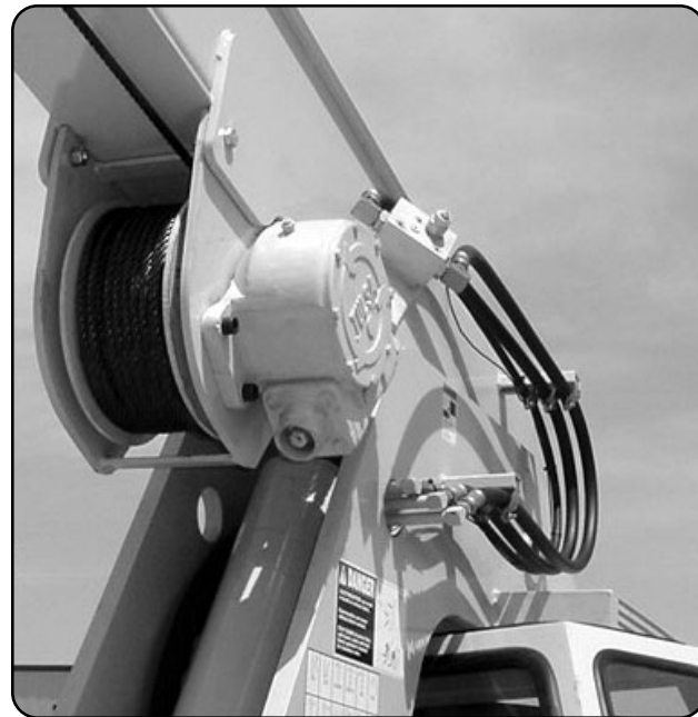
Large winch capacity for use with 1/2" (12.7 mm) wire rope
