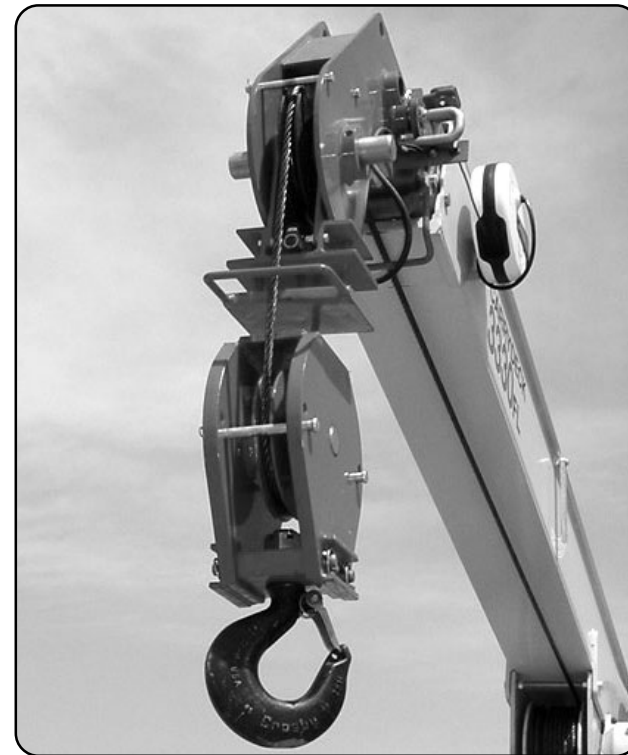
8.5 ton (7711 kg) lift capacity with 2-part line. Quick reeve main block for conversion to single line down haul block (tools not required).
