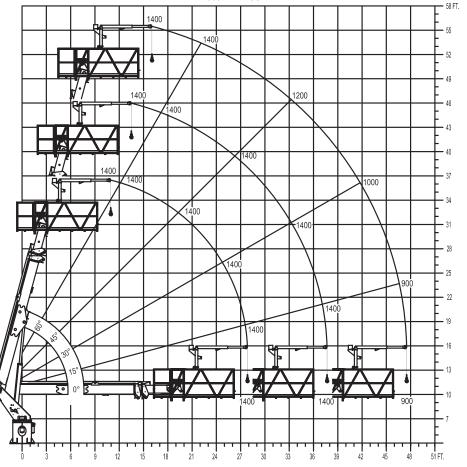
EXTENDED JIB 300 LBS. AT 45° AND BELOW AND EXTENDED JIB 500LBS. ABOVE 45° RETRACTED JIB 500 LBS. MAX. PERSONNEL 900 LBS. MAX.
