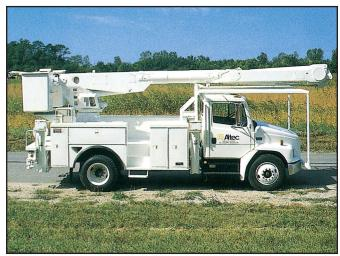
The AM650/AM855's side-by-side boom stow design offers low travel height with a low center of gravity and provides easy platform entry.
