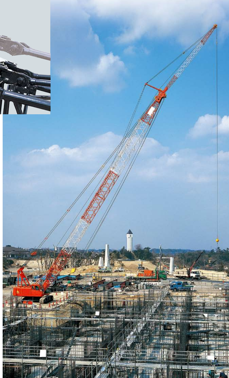
Bridge joint guides adopted for increased ease of boom disassembly and reassembly
