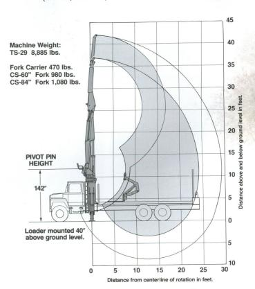
Figures shown here represent maximum hydraulic lifting force available at boom tip for each working radius at various elevations. Figures are maximum possible. Actual lifting capacities will vary with applications and actual worksite conditions. Deduct weight of grapple for payload.
