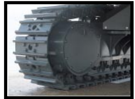
Sturdy guards shield the travel motors against damage from rocks.
