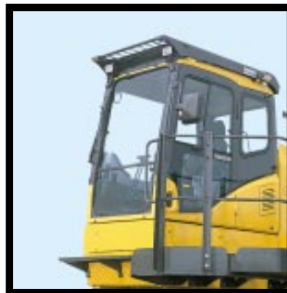
Photo shown includes Falling Object Guard (FOG).
