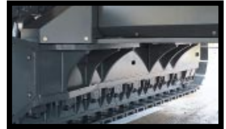
Sturdy guards shield the piping against damage from rocks.
