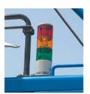
know operating conditions of "safety" or "marginal" or "overloading" with a 3-color of "green" or "yellow" or "red". As a further function, red lamp comes on automatically whenever operator cuts off LMI safety circuit absentmindedly.
