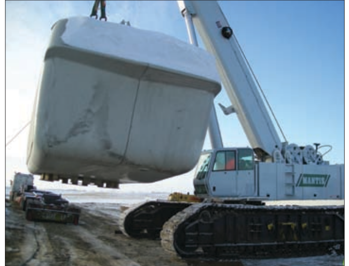
Full pick and carry capacity and long boom make the crane ideal for handling heavy turbine machine packages and long wind turbine blades.
