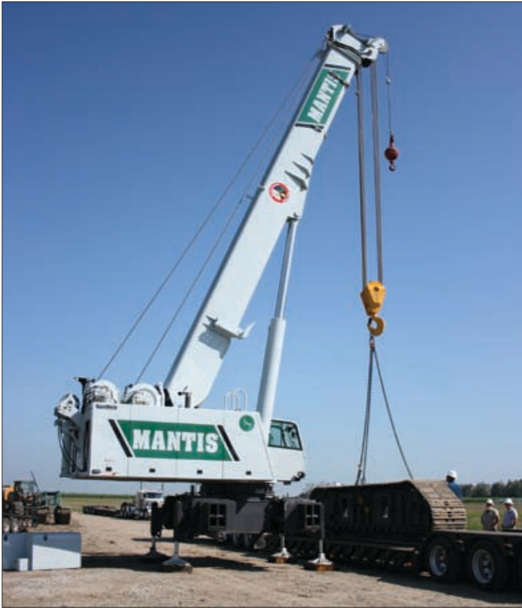
The GTC-900EX quickly and easily self-erects at job site.
