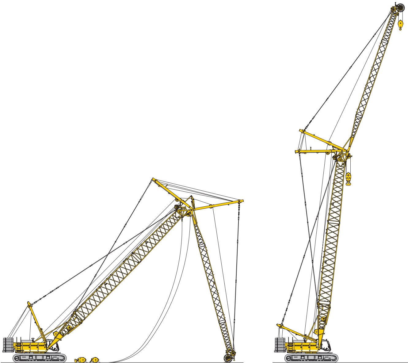
Erecting of main boom and luffing jib
