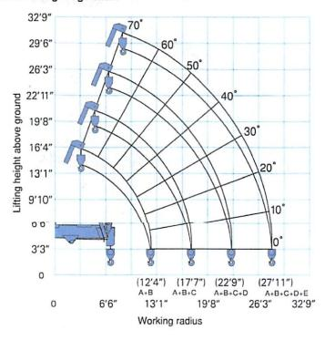
Working radius and lifting height are based on unloaded condition, excluding deflection of the boom.
