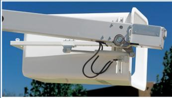
Non-Insulated Aluminum Inner Boom for increased payload and less wear and tear on chassis
