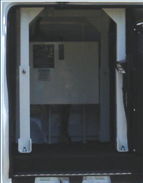
Remote Lower Controls provides great visibility for operation of the unit from the ground
