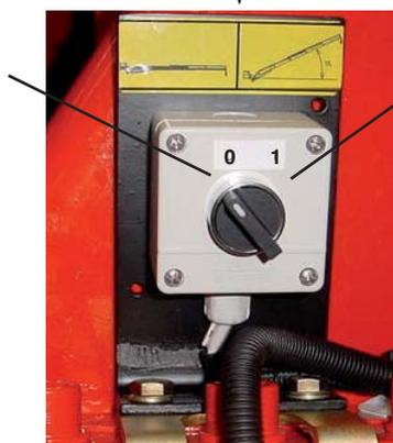
position of the selector when the jib is articulated at 25 degrees
