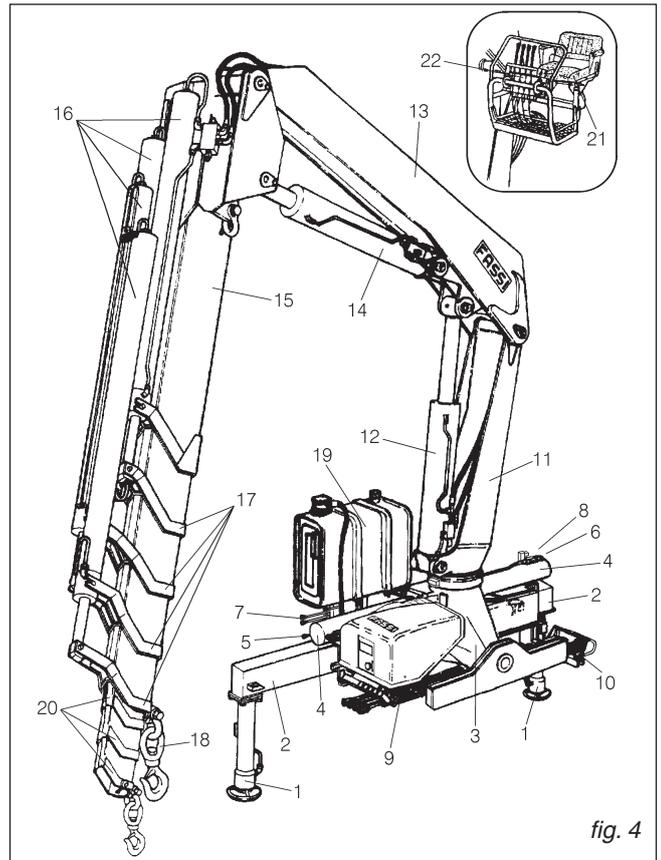
**9.2 Crane with top seat controls and with ground controls for outriggers. (fig. 5)**
