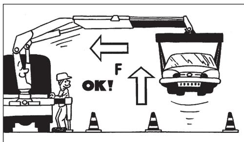
With vertical lift, on hydraulic and mechanical extension, rotate slowly in order to avoid side-skidding.
