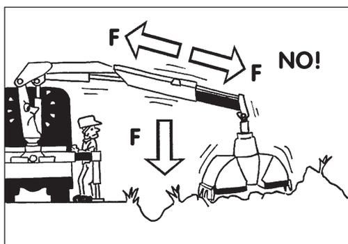
**(!) Never operate the outriggers when the crane is loaded.**
