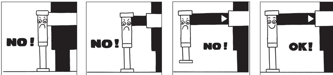
Remember that the stability of the unit (crane-vehicle) is only guaranteed by the complete lateral extension of the outriggers and by the observance of the capacity plates.
