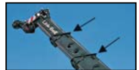
A-max extends only the inner-mid section of the boom for substantially increased capacities for in-close, maximum capacity lifts.
