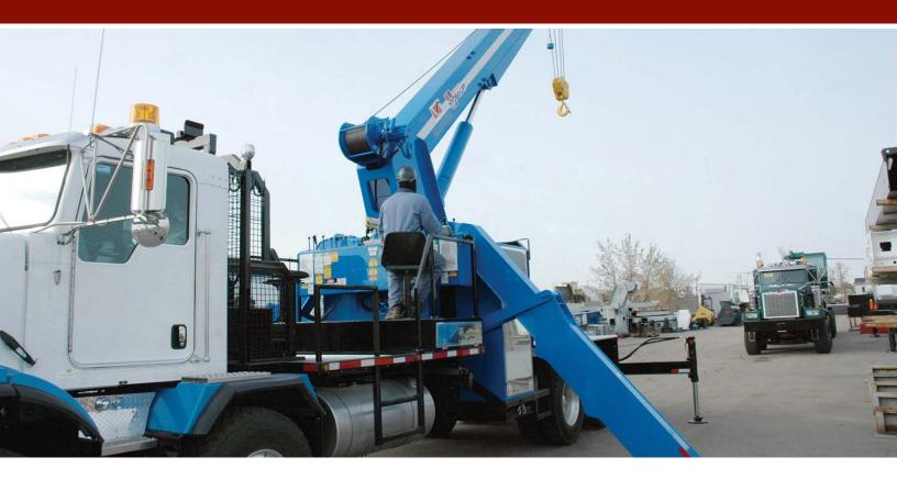
A 30-ton lifting capacity and short stowed boom length makes the HL30TC70 ideal for heavy work in the oilpatch. This crane can be mounted on either a single or double steering axle chassis.
