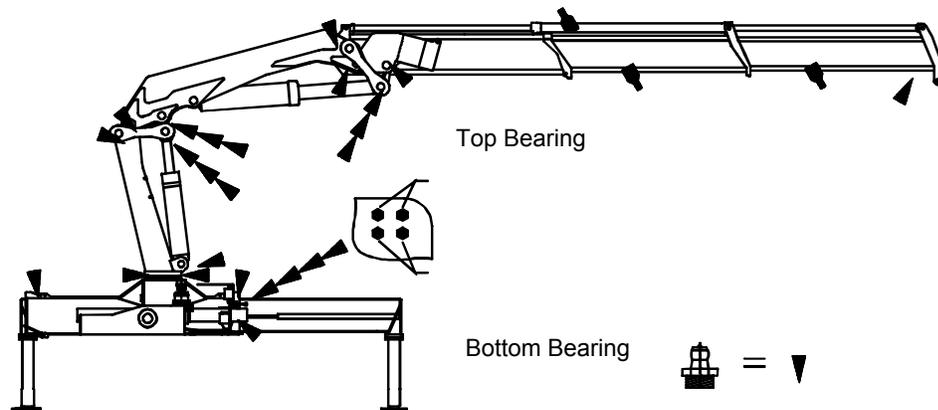
Example of a lubrication chart. For specific loader model, please see lubrication label on loader/Fly-Jib.
