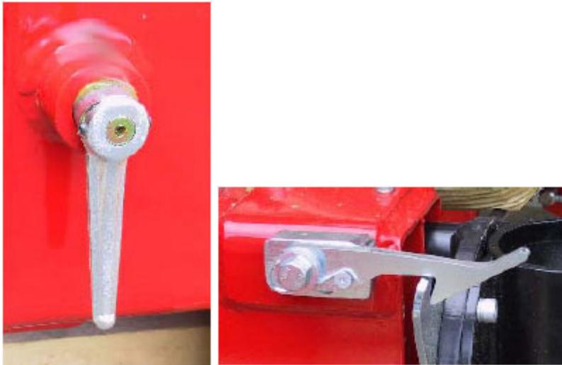
If the loader is equipped with swing-up outrigger legs they must also be secured in position before driving off. Before the vehicle is started, disengage the PTO and turn off the pump.
