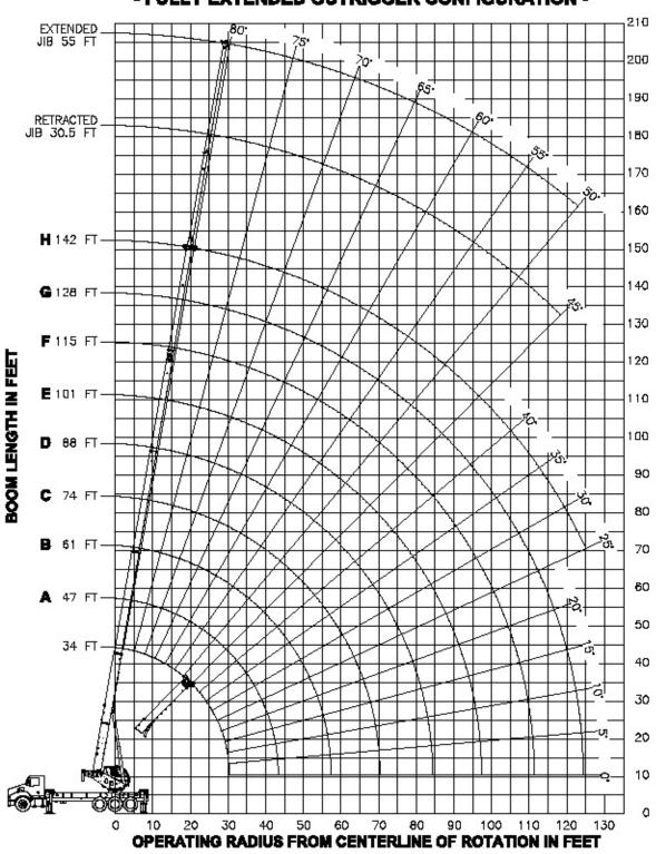
Lifting Capacities 5 section Boom 142 ft. 43,3 m Full Outrigger Extension
